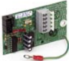
2XX-RS232 Additional bi-directional serial card 2XX-DN DeviceNet® option card
